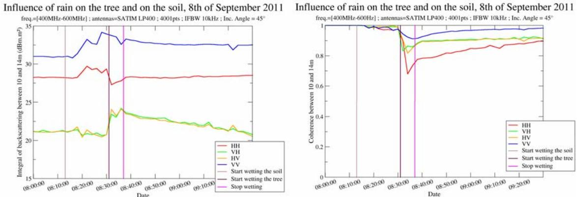
Figure 10. Evolution of the polarimetric intensity and coherence during the artificial watering.
