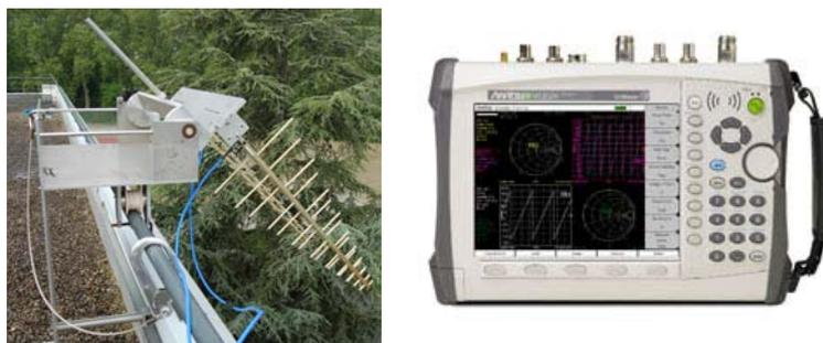
Figure 2. Mounting of the antennas on the roof and the VNA used for this experiment, respectively left and right.
