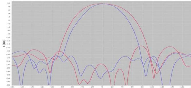
Figure 3. Radiation pattern in E and H planes, in co and cross polarization.
