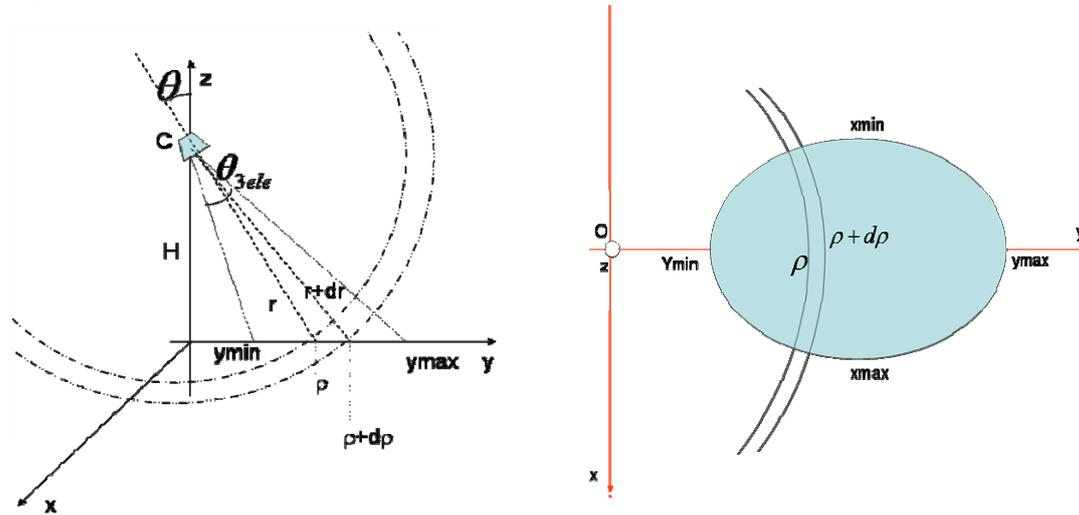
Figure 5 . Ground illumination after range gating; right: projection on the horizontal plane.
